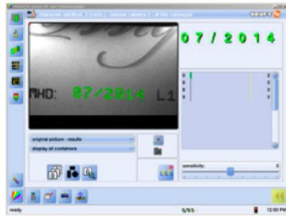
Are the labels present? Are they straight, without any offset and in the correct place on the wine bottle? Are they intact and without folds or dog ears? Is the label design really correct and in the correct language - does it correspond to the filled
