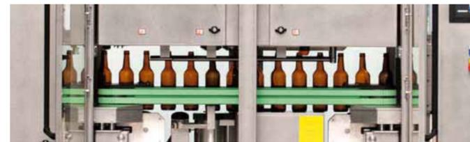
angle of rotation is implemented for each individual type of container; the bottles are correctly positioned and aligned at all the detection units. In addition the servo technology reduces the proportion of components prone to wear and makes product changes particularly fast and easy due to clearly reproducible brand adjustments. The intuitively understandable, audiovisual
