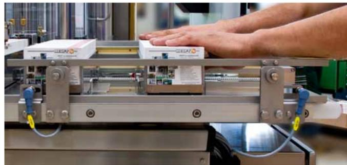
**Preventing cost-intensive standstills and saving human resources: this is also possible with the automatic magazine feed (AMF) for the HEUFT TORNADO W when wet glue labelling.**
