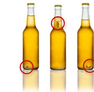
**The HEUFT eXaminer " XOS carries out a complete in-line inspection of full containers using optical and radiometric procedures. The new highly efficient HEUFT SPECTRUM " technology ensures that the detection of low density foreign objects functions just as easily and precisely as that of solid objects - in fact where space is limited.**
