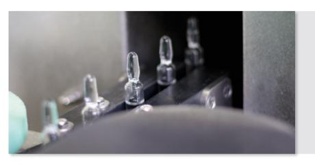
equipped with three CCD cameras for the complete inspection. The two below the conveyor belt carry out the base inspection and the two above the sidewall, neck and head or closure inspection. The ampoules or vials are each rotated by 120 degrees after every station in order to ensure a complete all-around inspection. The special arrangement of the servo-controlled belt drive effectively prevents faults being covered by it in the course of this.
